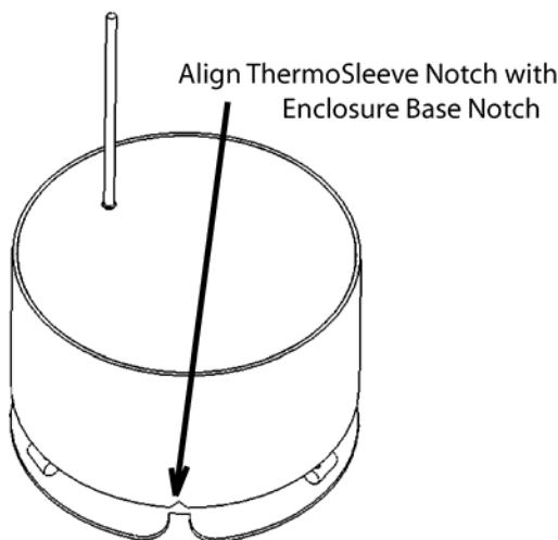
6. Check for full antenna extension by gently pulling on the antenna protruding from the ThermoSleeve.
