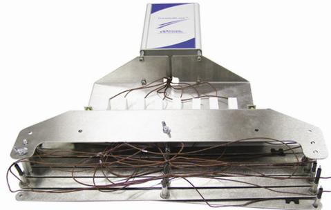
**TC-Bridge™** is a device designed to reliably position thermocouple probes while measuring temperatures in band ovens and freezer lines. TC-Bridge is easy to use since the factory routed thermocouples remain in place in both stowed and deployed configurations; the thermocouples simply fold neatly away as the device is stowed.
