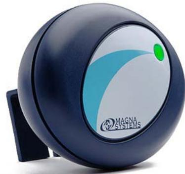
The GateWay is a high performance wireless network access point used with Magna Systems' measurement transducers and powerful DataLink™ software to implement test and measurement platforms. The GateWay manages and controls network communications including network initialization, transducer configuration, data collection, alarm condition management and network diagnostics. The USB 2.0 compliant PC interface provides high speed connectivity and power for the GateWay.
