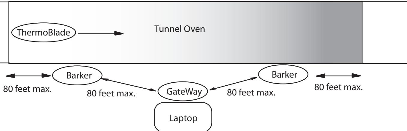
Step 1. Position Barkers at specified locations per the Barker installation diagram
